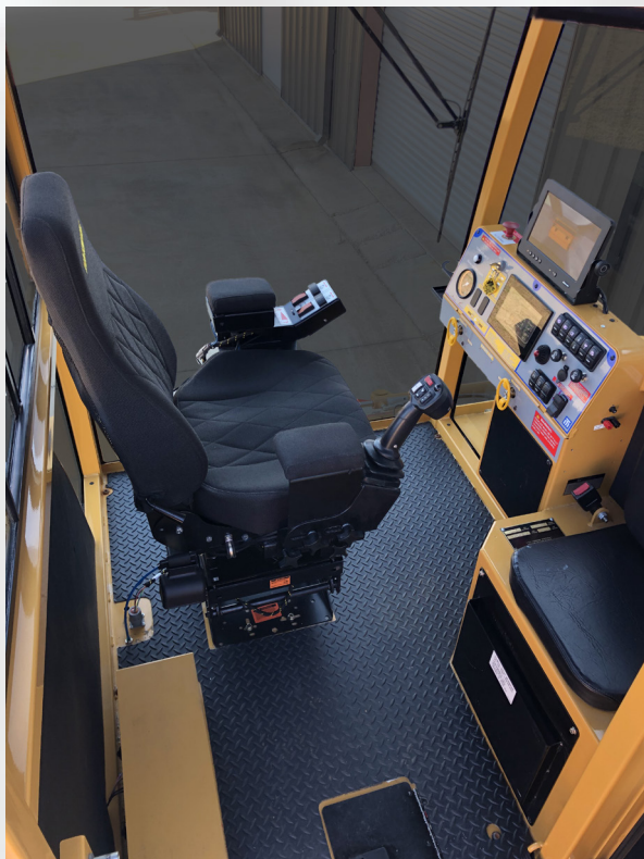
Spartan control panel and operational controls.
